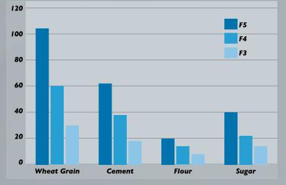
The graph demonstrates the throughput in tonnes per hour for product handled by the range of Floveyor  $^{\scriptscriptstyle \rm TM}$  machines.
